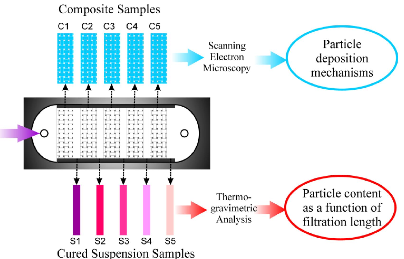
No clay filtration could be observed by visual observation of the samples, at any fiber volume fraction. Glass microspheres were partially filtrated when 27% fiber volume content was set, leading to a deep filtration mechanism. When a fiber volume content of 47% was set, glass micro spheres could not enter into the microstructure of the fabrics, thus surface filtration occurred.
